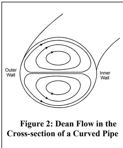
**Figure 2: Dean Flow in the Cross-section of a Curved Pipe**
