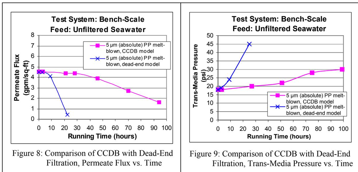
polypropylene melt-blown cartridge. The CCDB system provided a service life about five times longer than the conventional dead-end system with the same type of filter media installed. The SDI level for the permeate was measured to be between 4.7 and 4.9 in this test.
