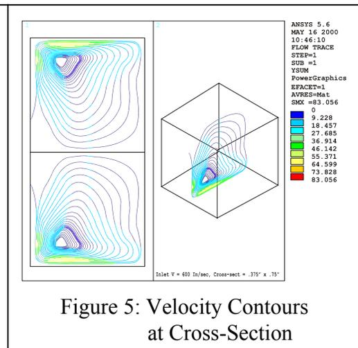
is generated as the processed fluid flows through the spiral passageway. The vortex currents in the spiral passage provide high shear filtration across the filter surface to remove the debris trapped on the surface and transport it away, resulting in superior fouling control.
