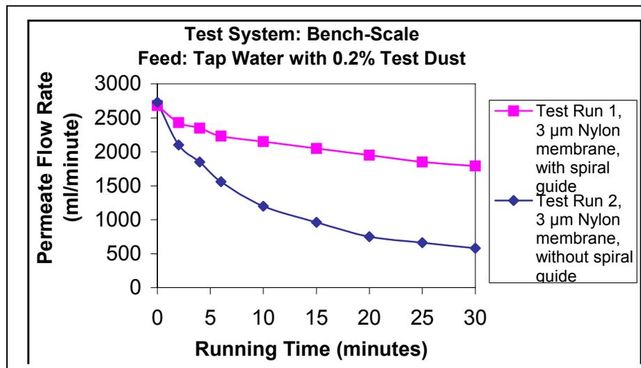
second for trials lasting approximately 30 minutes. As seen in Figure 7, Test Run 1 employing a spiral guide maintained a superior permeate flow rate throughout the trials as compared to Test Run 2 where no spiral guide was present. The permeate flow rate also degraded less for Test Run 1.
